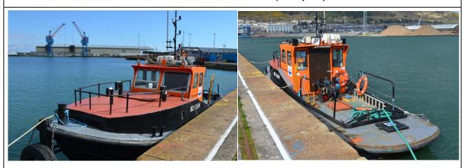
The 'Boy Euan'. is a 12.6m x 3.25m Steel hull, highly manoeuvrable, single propulsion type workboat. The vessel has a multiple of uses and is fully certified by Mecal. Category 3 - 20 miles from a safe haven. The vessel is designed with towing in mind with a large clear deck aft also suitable for carrying equipment. Available for hire or charter and comes with a fully qualified crew. The vessel is fully road transportable and can be transported via a low loader to any site.
