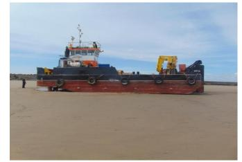
FUEL TANKS: 4no 18m3 plus 4no 15.9m3 FUEL TRANSFER: 100m3/hr - 1.5 bar FRESH WATER TANKS: 2no 13m3 & 1no 16.5m3 FRESH WATER PUMP: 25m3/hr - 1.5 bar FRESH WATER CAPACITY: 40,000 Ltrs
